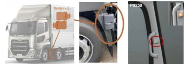
BSIS and LCS radars location on the QUON
