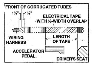
5. Secure the front of the corrugated tubes to the wiring harness with electrical tape as shown in the figure on the left.
