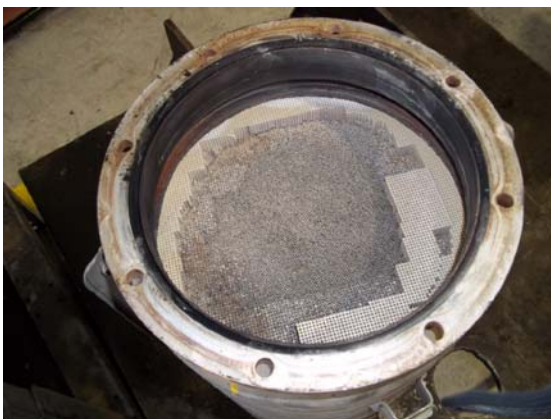
Major Ceramic Substrate damage
