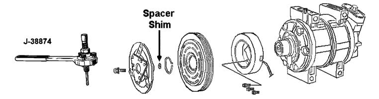
Refer to the Air Conditioning section of the appropriate Service Manual whenever it is necessary to replace the magnetic clutch assembly.
